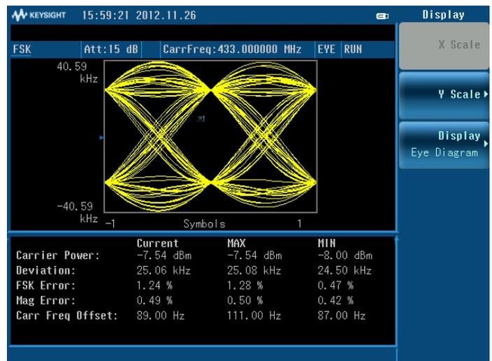
Figure 6. FSK demodulation with eye diagram view
